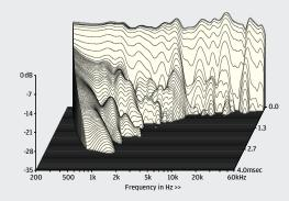
ABOVE: The compact cabinet is well damped while only low-level modes are seen from mid and ribbon
